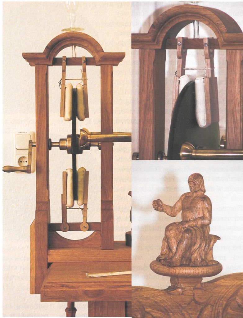
Fig. 8. Details of the replication of Schmidt's electrical machine (side view, the cushions and a carved figure of Zeus).
