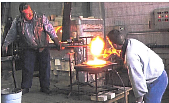
Fig. 6. Casting the glass plate in a heated mould made of steel in a workshop in Gehlberg.
