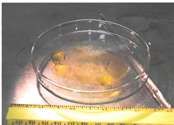
Fig. 10. Traces of gold film just forming on the bottom of the Petri dish.
