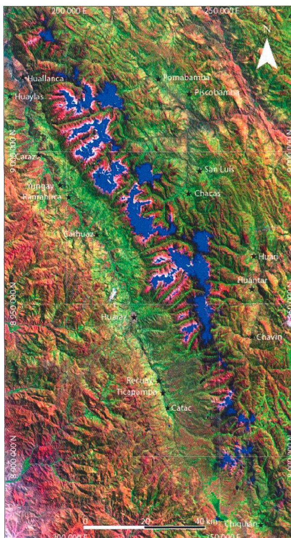
Fig. 3. Ratio image (2010) TM4/TM5 \geq 2 showing Cordillera Blanca glaciers (blue). Background: composite image of Landsat 5 TM of 18 August 2010 (RGB: 7/4/2).
