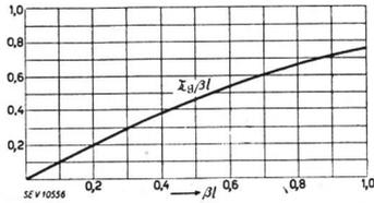
$$\mathfrak{T}_g \beta l = \beta l - \frac{1}{3} (\beta l)^3 + \frac{2}{15} (\beta l)^5 - \frac{17}{315} (\beta l)^7 + \frac{62}{2835} (\beta l)^9 - \dots$$
