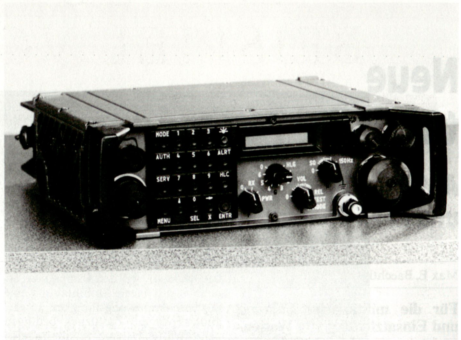
Tragbare 4-Watt-Station PR4G (Poste Radio 4 e Génération)
