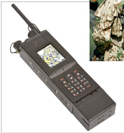
© Thales Software Defined Radio Handheld Terminal (V/UHF) interoperable mit LTE™ Terminal TESquad dank Unified Networking (© Thales NEXIUM Theatre).
