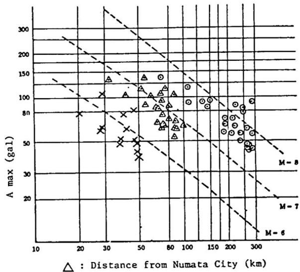
Fig.4 Relation between the Earthquake Focus and Acceleration
