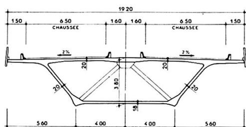
Fig. 12 - Section transversale
