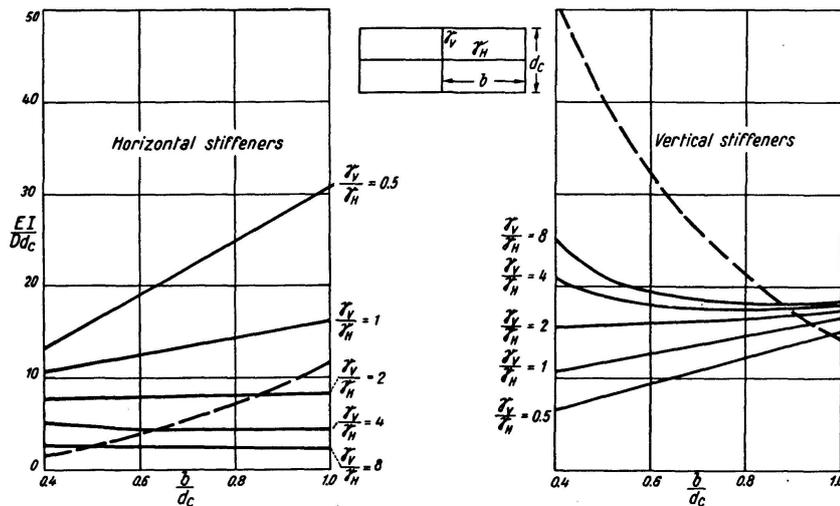
Fig. 8. --- Empirical Relationships. Equation 3 for Vertical Stiffeners. Equation 5 for Horizontal Stiffeners. — Design Law in DN 4114<sup>12</sup>.
