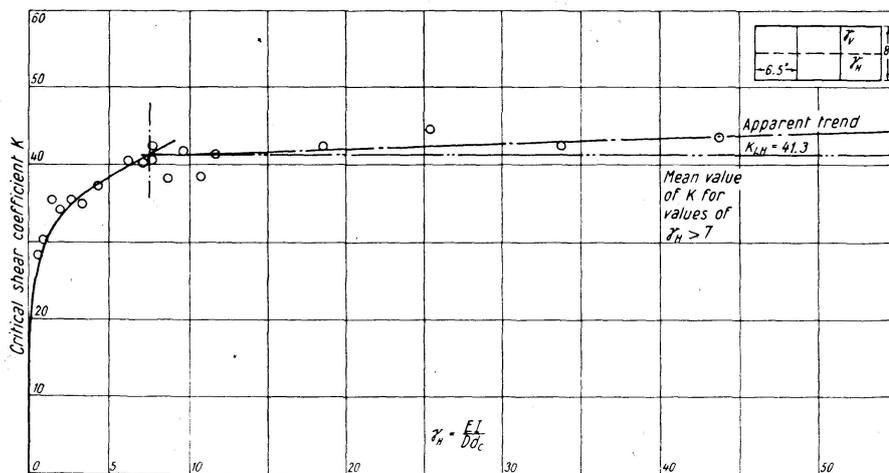
Fig. 3. Results Obtained with Vertical Stiffeners at 6.5 in. Centres on Webplate Having Clear Depth  $d_c$  of 8 Ins.  $\gamma_v$  of Vertical Stiffeners 93.5. Varying Size of Horizontal Stiffeners.
