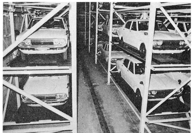
Automated warehouse (Nissan Motor Co., Ltd.)
