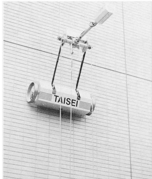
Photo 22 Tile inspection robot
