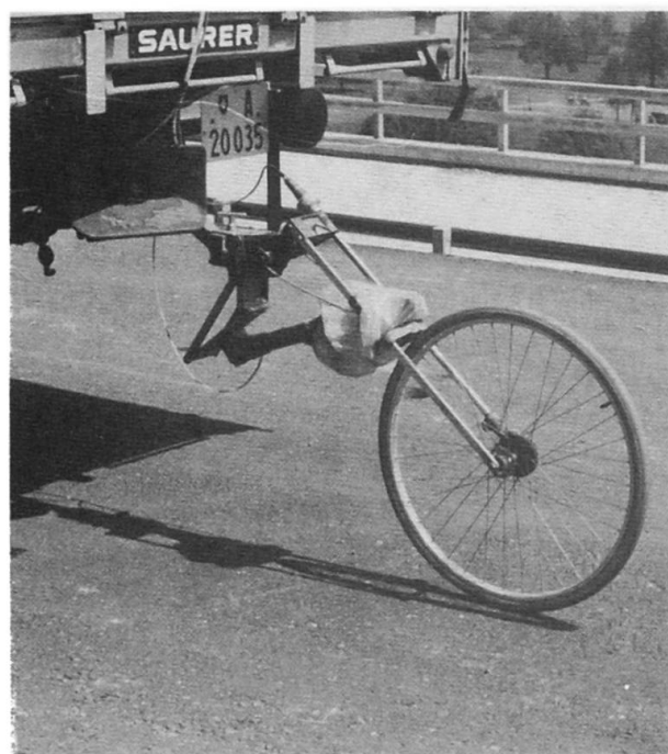
Fig. 4 With the help of a test wheel, the speed can be accurately measured and controlled during the passage.
