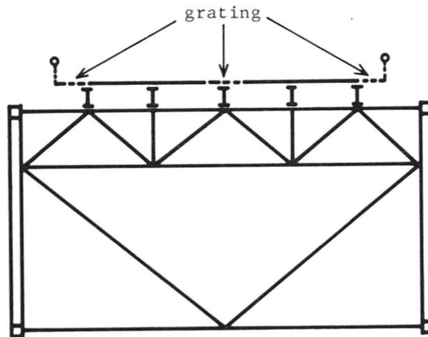
Fig. 10 Cross section of stiffening truss
