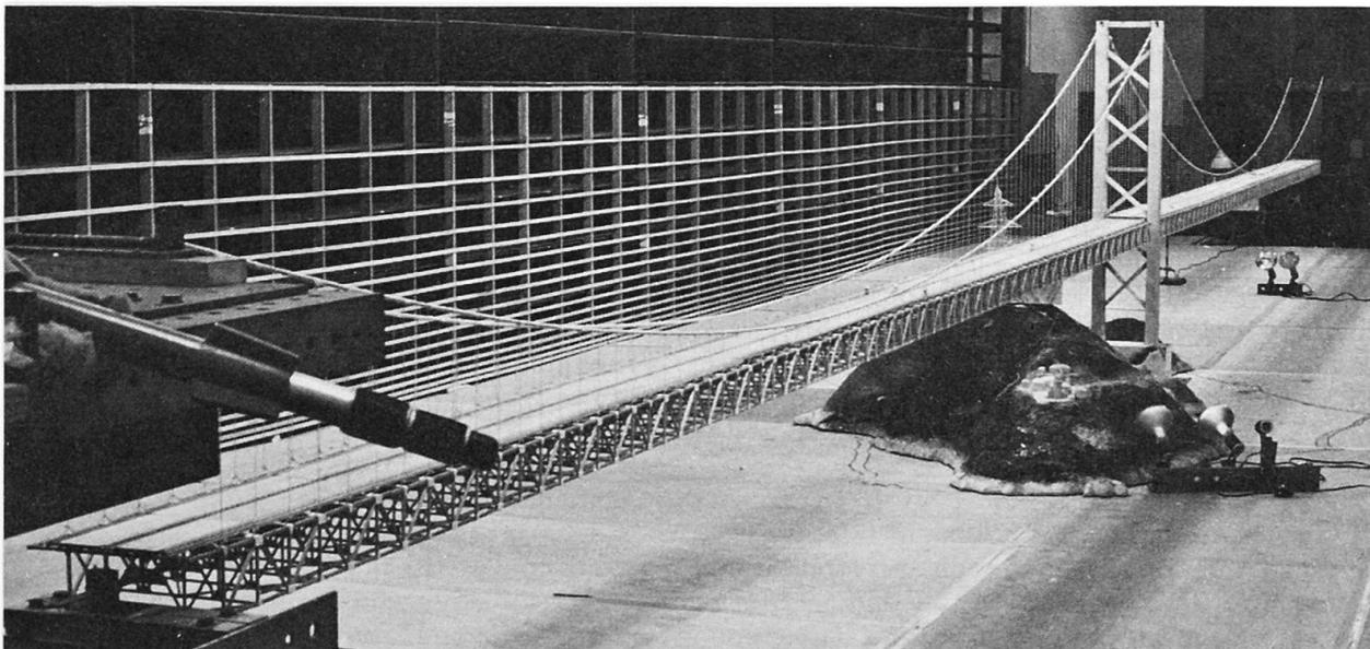
Fig. 12 Suspension bridge full model in wind tunnel
