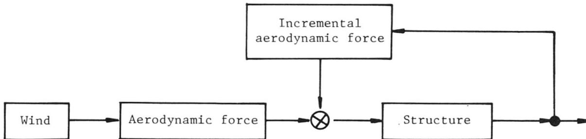
Fig. 1 Block diagram illustrating the onset of flutter
