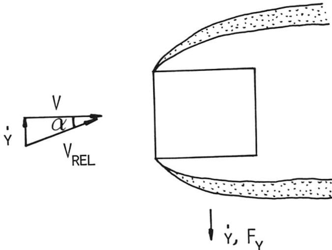
Fig. 3 Section and flow geometry for the quasi-steady analysis of galloping
