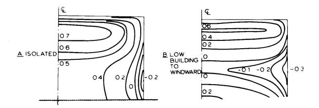
2. Pressure distribution on the windward face of a slab block (a) in isolation (b) with a low building to windward. (67.479.3)
