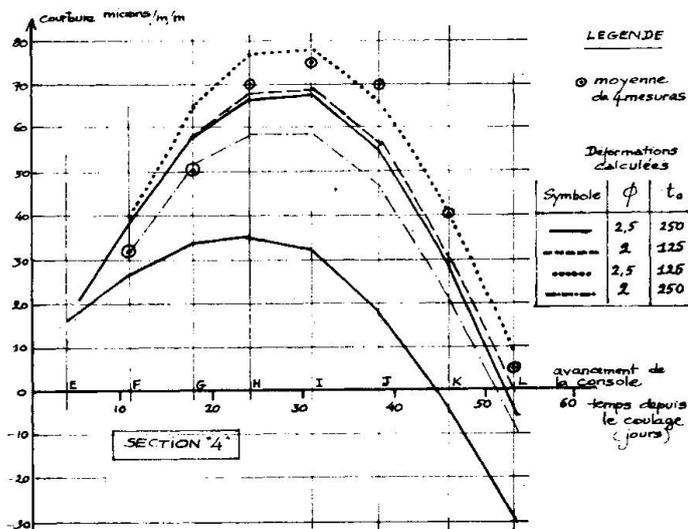
FIG. 3 COMPARAISON DES COURBURES CALCULÉES ET MESURÉES
