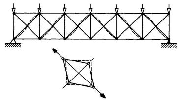
The diagonals in compression are buckled under load and only diagonals in tension are working.
