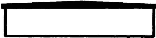
Tapered Beam Width: 28' through 80' Height: 10' through 20' Slope: 1:24
