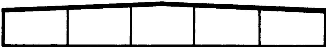
Beam and Column Width: 48' through 400' Height: 12' through 30'
