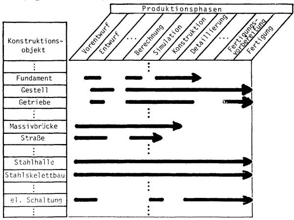
The horizontal axis shows the various phases, which must be passed through in design, calculation and manufacture; typical engineering subjects are listed vertically. The tasks to be dealt within production are plotted in fig. 1 as horizontal lines, each associated with the related subject. Depending upon the engineering aspects or the particular features of the firm, there may be breaks in a line, since all the phases are not relevant to every case.
