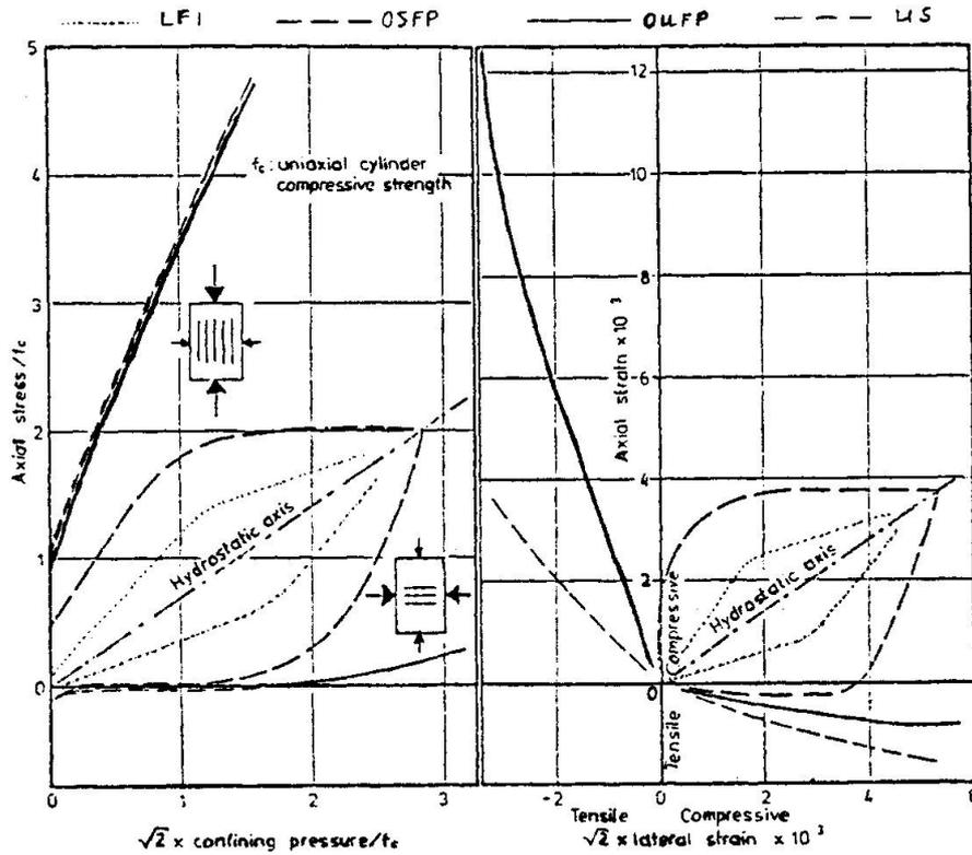
Fig. 6 Failure envelopes for concrete as derived from triaxial tests data for cylinder
