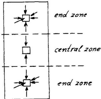
Fig. 7 Schematic representation of the effect of boundary frictional restraint on the state of stress within cylinders
