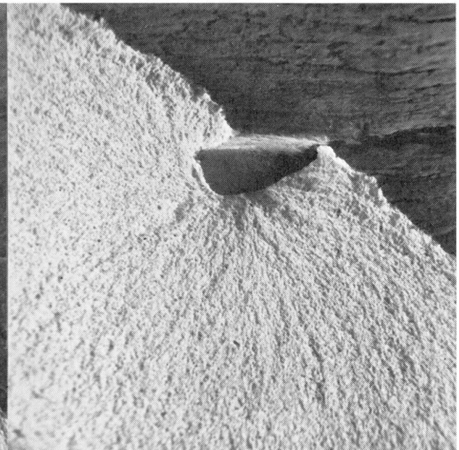
Fig. 5 steel III b, cold-worked Small delamination defect, initiation at high stress level:
