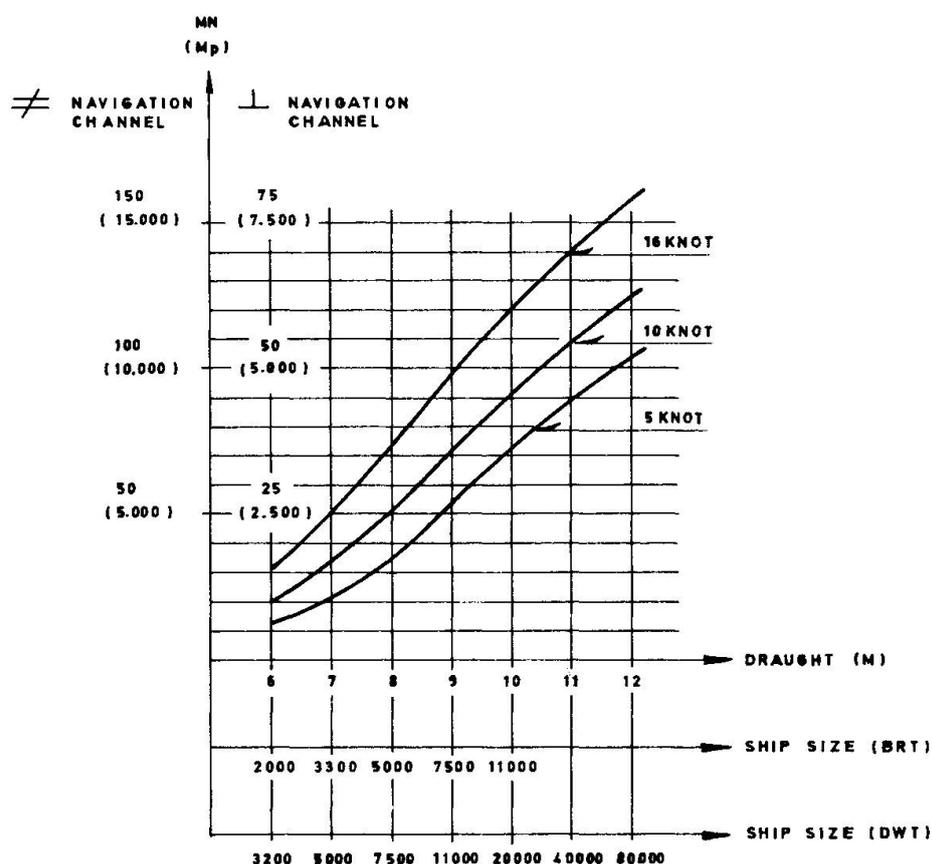
**Fig. 4** Magnitude of ship collision force as a function of ship size and speed. (From [8]).
