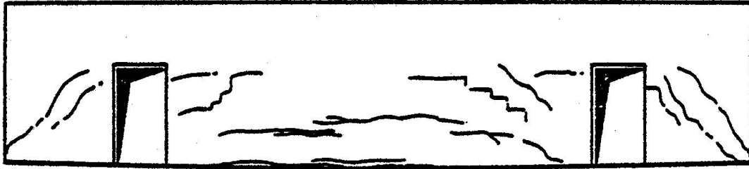
Fig. 2 Significant cracks in a masonry partition supported by a flexed beam
