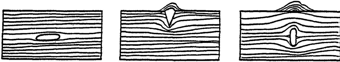
Fig. 17 Variation of magnetic field due to defects in steel
