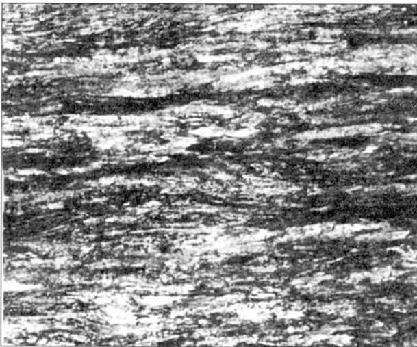
Fig. 10 Micro-Structure of a Galvanized Wire (400 Magnifications)
