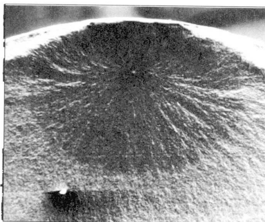
Fig. 7 Fatigue Fracture Surface of an OT Wire (50 Magnifications)
