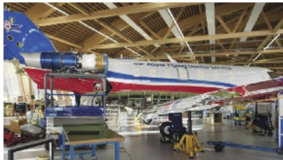
A PC-24 destined for the Australian Royal Flying Doctor Service being assembled in Stans.
