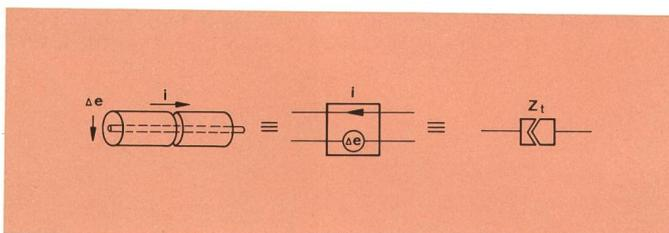
Fig. 1 Screening effectiveness circuit for definition of  $Z_t$
