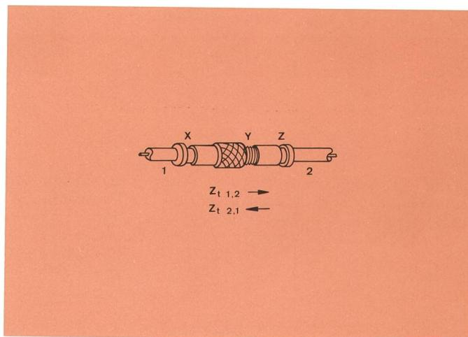
Fig. 2 Real connector assembly with the possibility of  $Z_{t1,2} \neq Z_{t2,1}$
