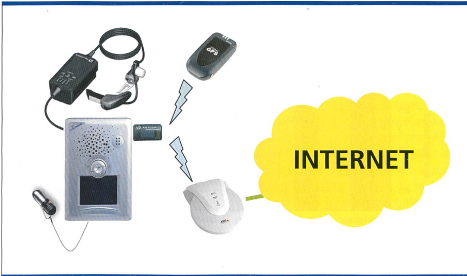
Fig. 2. Prototype of a smart assistant on a small PC with wearable end-devices.
