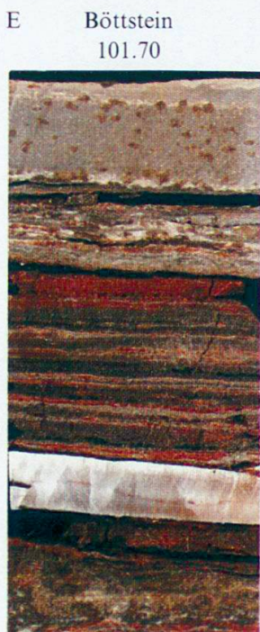
101.92 Anhydritized porphyro- blasts in arenite and satin spar gypsum vein. Gipskeuper III C
