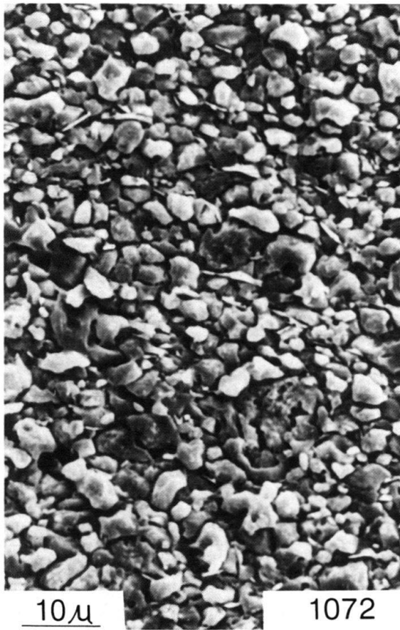
Fig. 9. SEM micrographs obtained from etched polished surfaces showing typical microstructure of sample 1072 from the anchimetamorphic Helvetic Nappes.
