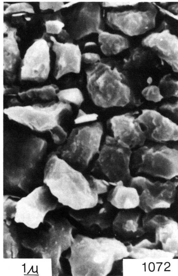
Fig. 9. SEM micrographs obtained from etched polished surfaces showing typical microstructure of sample 1072 from the anchimetamorphic Helvetic Nappes.
