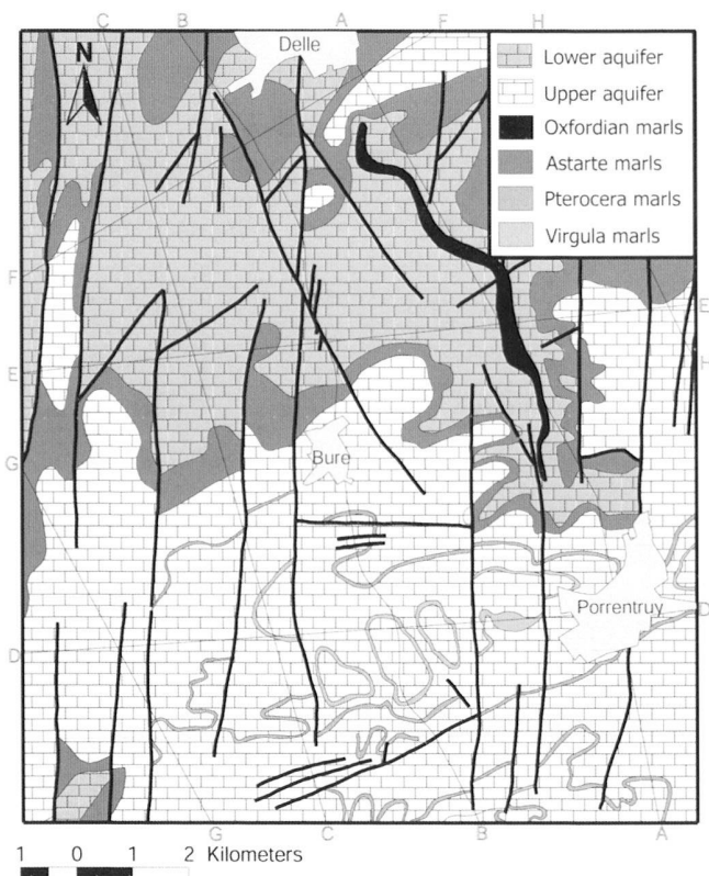
Fig. 4. Hydrostratigraphic map. Tertiary and Quaternary sediments are omitted. Marl levels are indicated for orientation. Malm limestones are merged for simplicity. Thick lines mark tectonic features; cross sections are indicated by thin solid lines.
