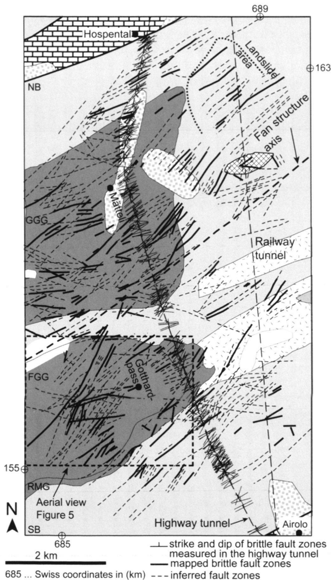
Fig. 3. Fault zones mapped in the area of the Gotthard pass. Black lines represent mapped brittle fault zones, dashed lines represent inferred fault zones based on aerial photos and geomorphological mapping. Strike and dip of mapped brittle fault zone within the Gotthard safety tunnel. See Fig. 2 for legend.
