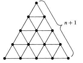
This array is called the *(big) hive triangle*. When lines are drawn through the hive vertices as shown, the hive triangle is split up into  $n^2$  small triangles. By a *rhombus* we mean the union of two small triangles next to each other.
