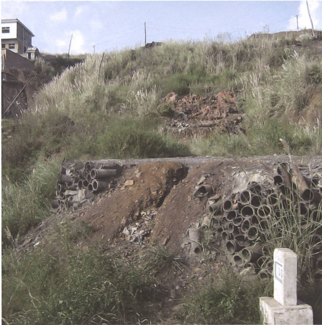
3 (B) Abandoned zinc retorts in Hezhang County, Guizhou Province, China.
