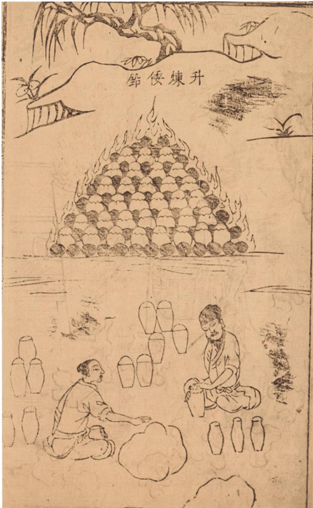
3 (A) Illustration of a zinc-smelting scene in the Tiangong kaiwu 天工開物 (Exploitation of the Works of Nature, published in 1637).
