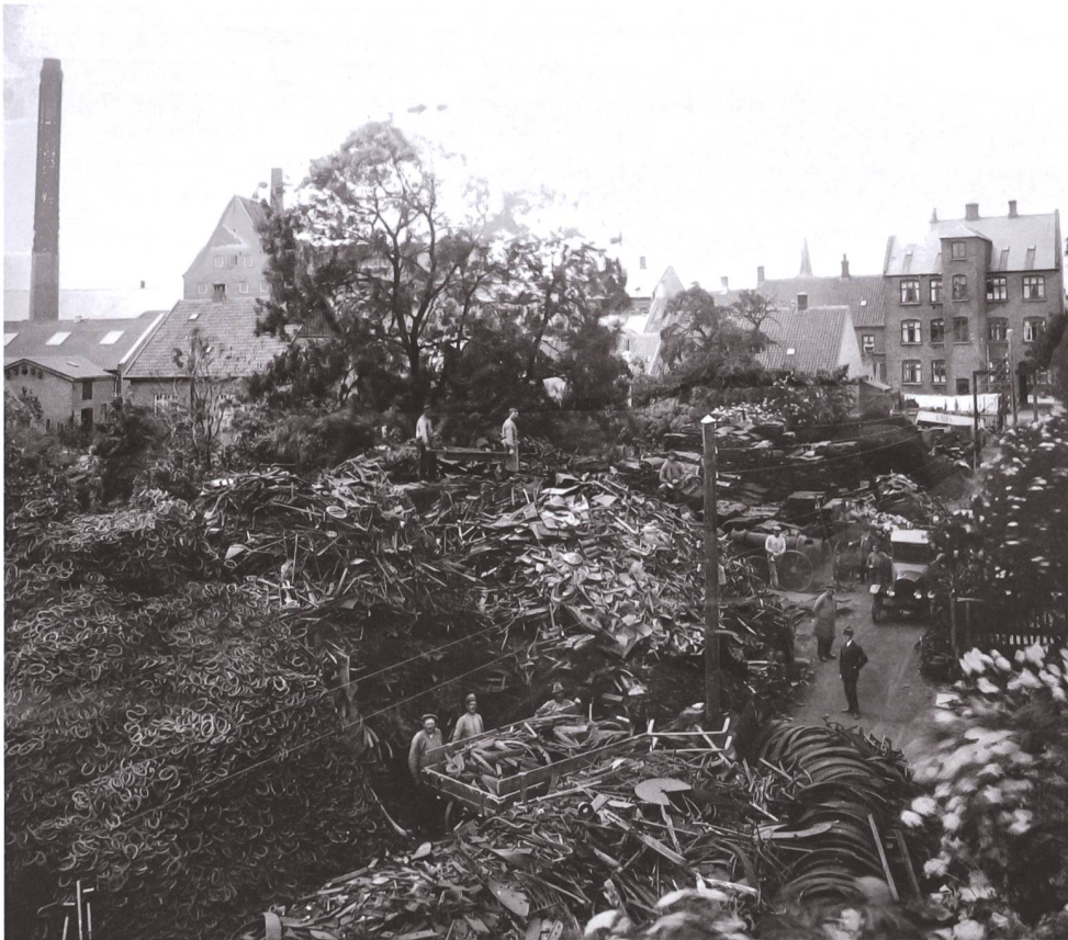
4 The yard of one of Denmark's largest scrap companies in the mid-1920s. Even then, the scrap had to be sorted carefully. For example, the pile on the left consists exclusively of horseshoes.
