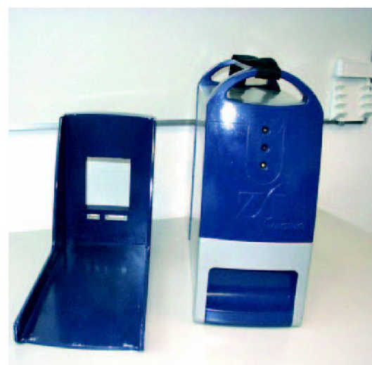
Fig. 4: flight data storage unit FDS.
