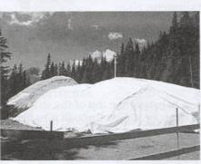
of snow into a seven-metre high pile. Half was covered with fleece and half with a 40cm layer of sawdust.
