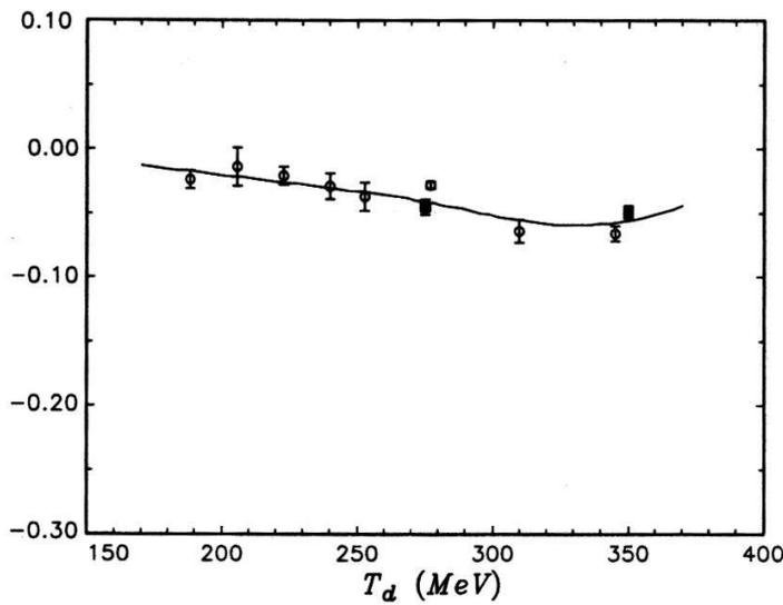
Figure 1: Polarimeter effective analysing powers  $iT_{11}$ ,  $T_{21}$  and  $T_{22}$ . Open circles : this experiment; Crosses : ref. [8]; Full squares : ref. [10]. The curves are the results of the polynomial fits.
