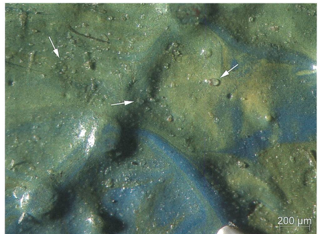
Fig. 20 Landschaft mit Reiter auf Brücke : detail in the meadow under the trees; the layer of varnish is extremely thin. Examination with a stereobinocular microscope reveals the presence of transparent inclusions (particles indicated with white arrows).
