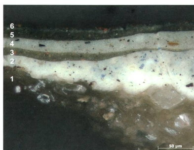
Fig. 4a In visible light. Layer build-up: 1 ground layer; 2, 4, 6 opaque layers; 3, 5 glazes. (Varnishes not indicated.)
