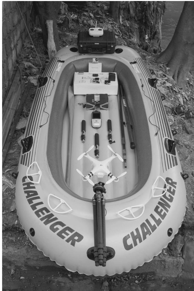
Rubber boat, GoPro action cameras, DJI Phantom quadrocopter, FARO Focus3D high-speed 3D laser scanner, Trimble GeoXH handheld Global Navigation Satellite System. In Kampung Melayu, Jakarta, Indonesia, 2013.
