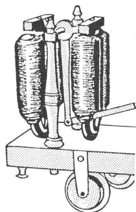
Fig. 3 Motor von G. O. Coltons Lokomotive, 1847 [1]
