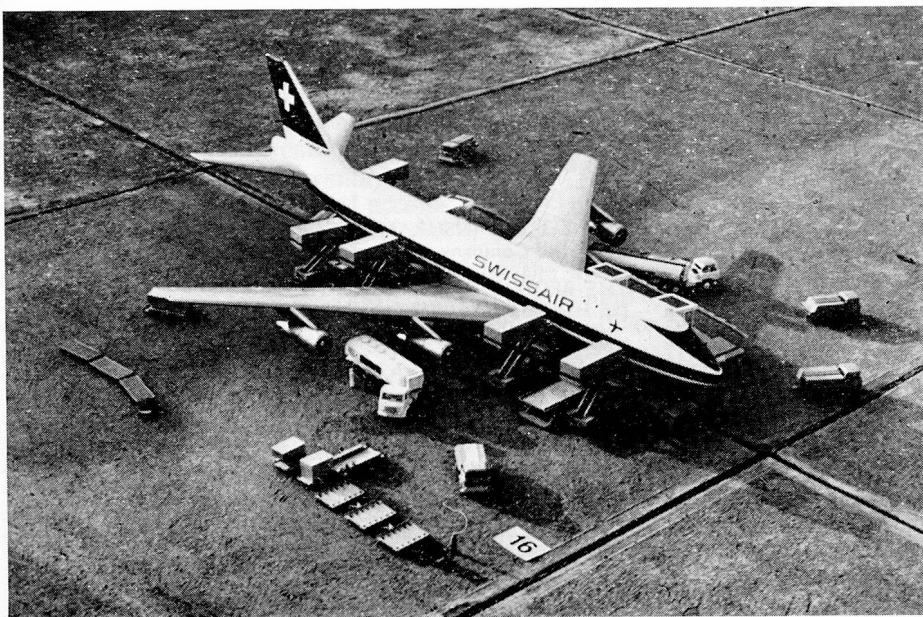
Swissair is at present using models to study the ground handling problems associated with the Boeing 747B "Jumbo" jets which it has on order. More than 20 vehicles will be involved in the departure of a single Boeing 747B including a 50-ton tractor.
