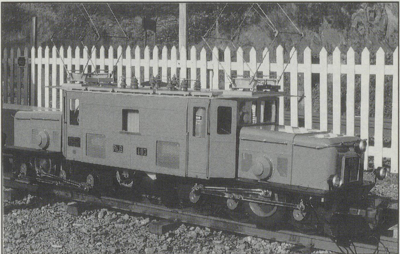
Pfeifferbahn built the mechanical parts and supplied the electronic control gear. The customer built the bodywork from wood (except the two bonnets, for which he obtained the services of a maker of replica armour!) Finally, all the electrics were assembled and tested on site by a friend of the customer.
