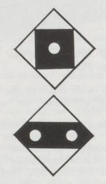
At unstaffed halts, a passenger operated flashing light is located at the braking distance from the halt. The original type consists of a single white light with a square black surround on a larger white diamond-shaped background whilst the later type (GFM and others) has two alternately flashing white lights on a black bar on a white diamond.
