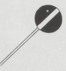
Portable STOP signs take the form of a red disc with a white bar by day. At night a red lamp is hung from the disc.
