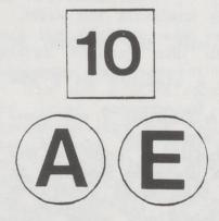
The beginning of a rack section is preceded at a distance of about 150m by a square white board with black numerals, giving the speed allowed on that section. The beginning of the rack rail is marked by a round white board with a black letter A (C in French-speaking areas), and the end of the rack rail by a similar board with the letter E (F in French). The two indications are usually on opposite sides of the same post.
