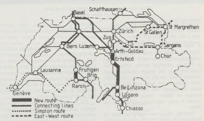
The sketch map above is derived from one which appears in issue 2/92 of the SBB Magazin, showing, diagramatically, the various routes that will be upgraded in connection with the new deep level basis tunnels under the Gotthard and Lötschberg. Our map in the September 1990 issue of Swiss Express gives rather more detail of the proposed tunnels.
