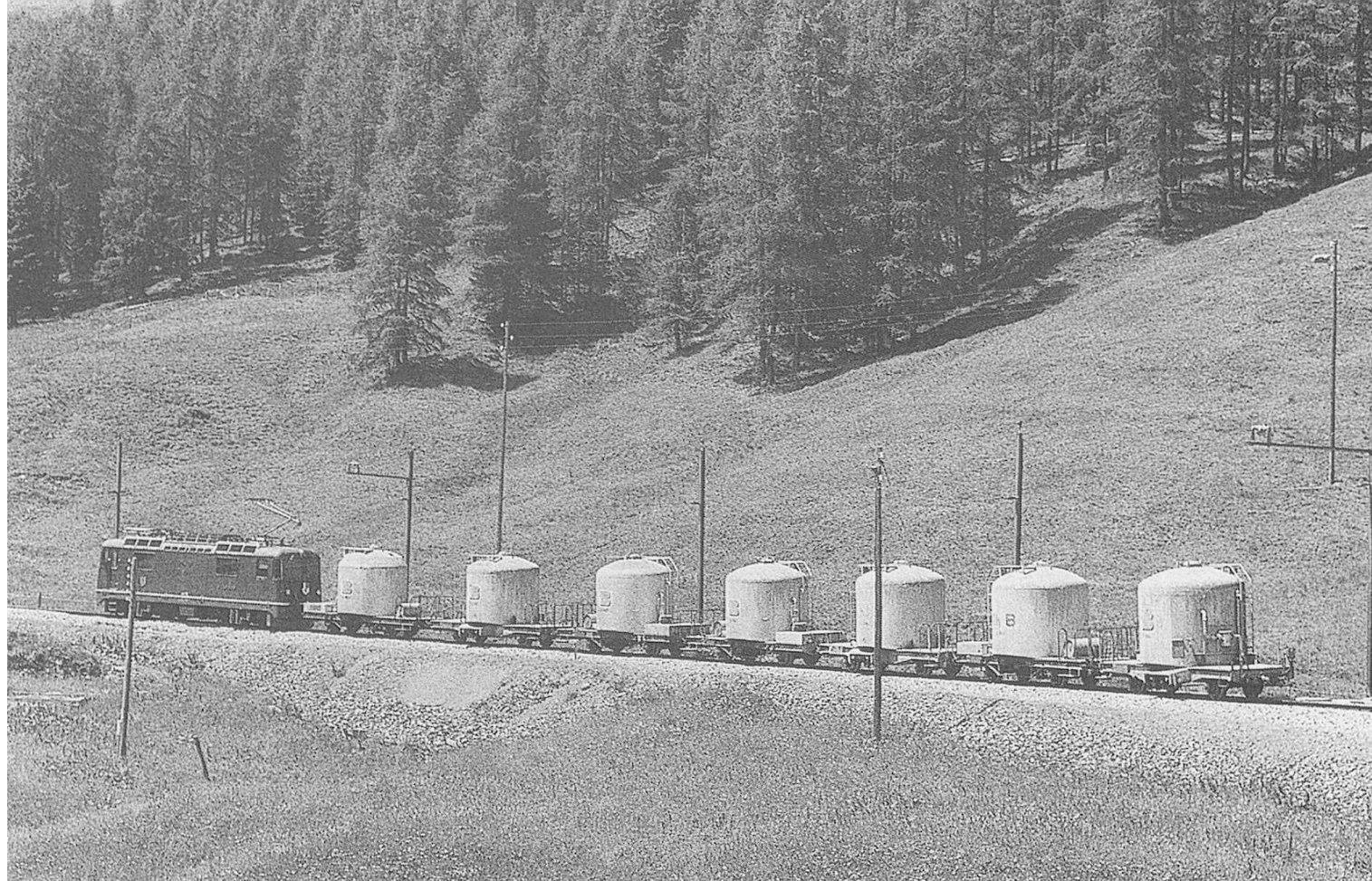
A cement bulk freight train on the 45‰ ramp below Davos Wolfgang hauled by a Ge4/4II on 23 June 1978
