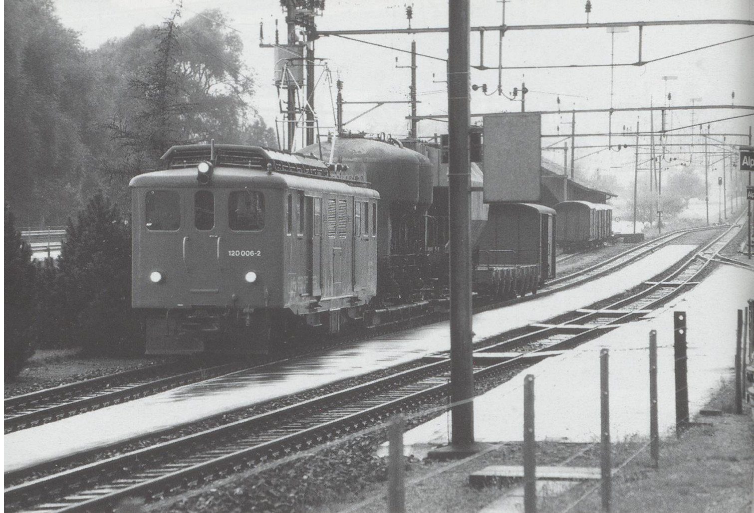
Above: Deh 120 006-2 at Alpnachstad with a standard gauge cement wagon on a rollschimmel wagon and metre gauge goods wagons..
