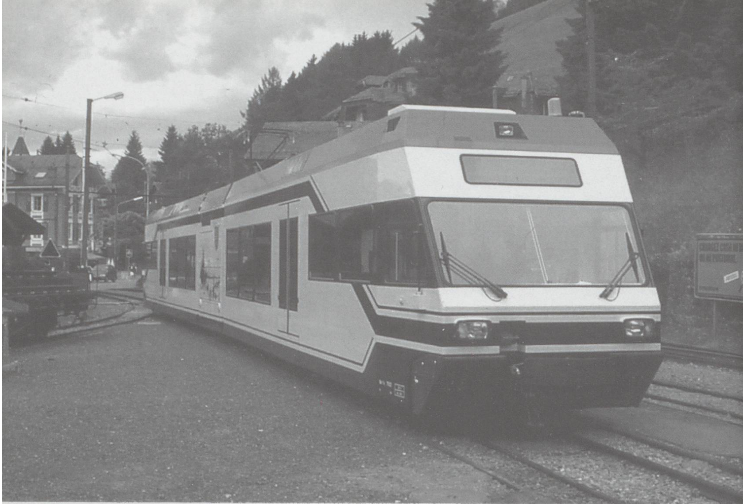
Above: MOB Be2/6 'push-pull' articulated unit at Les Avant, 10/6/98.
