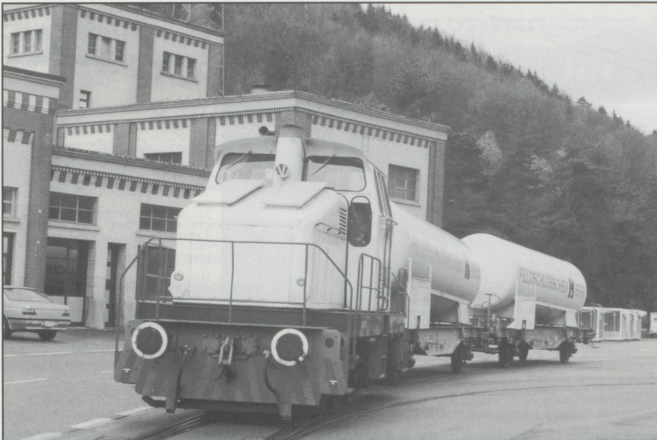
Shunter wagons loaded with demountable road tanks waits at brewery. Public road behind locomotive. April 2000
