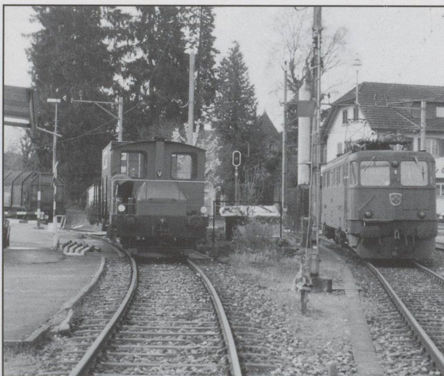
Reinach in April 2000. The tractor is being refueled from a drum and an Ae 6/6 waits for the coil wagon to be unloaded.
