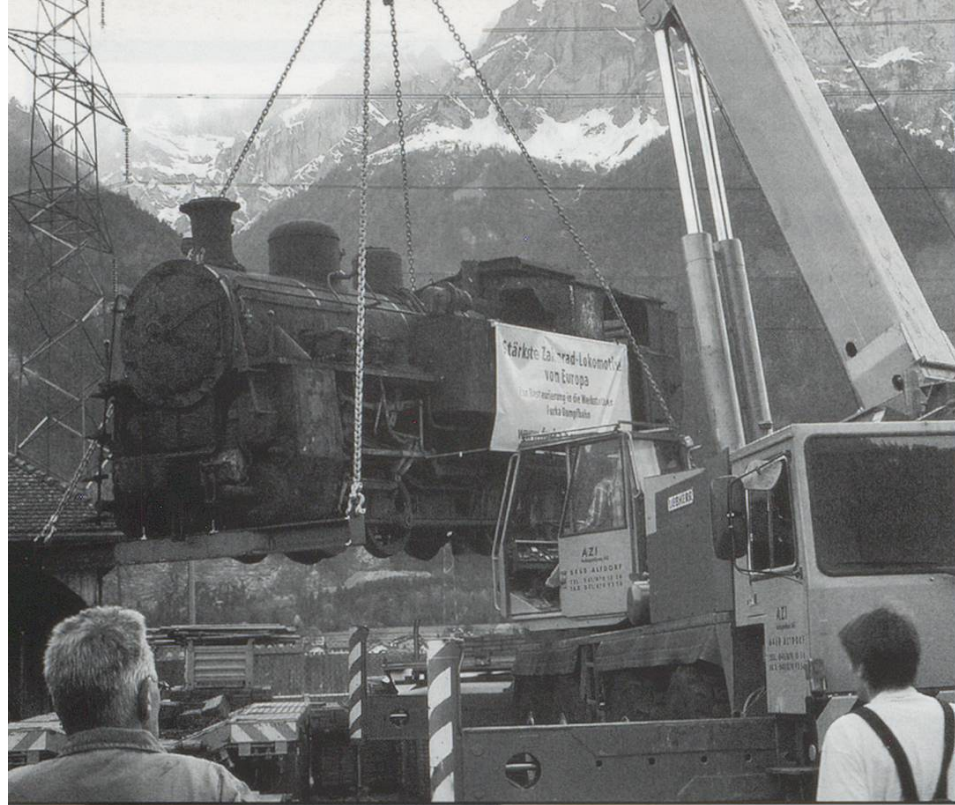
LEFT: The crane lifts the locomotive onto the trailer at Altdorf
